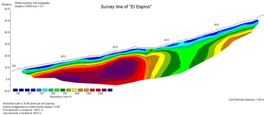
Figure 3: Resistivity profile across the survey line after topography corrections and 5 iterations in the inversion program, for a RMS error of 2.1%. The black line represents the inferred fault. The resistivity values are shown in a logarithmic scale.
