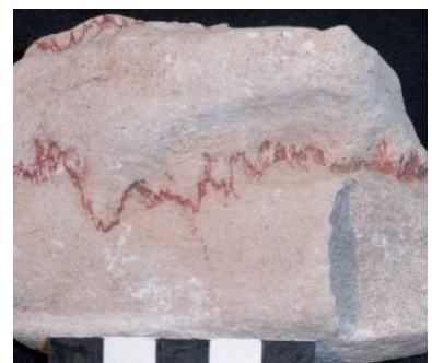
Figure 8.5 Stylolite picked out in white limestone by red, insoluble iron oxide. Scale = 5 cm. (Tom W. Argles, The Open University, UK.)
