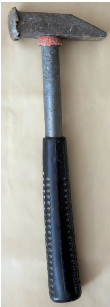
Figure 2.20 Geological hammer with head showing spalling (head is 12 cm long). Further use is likely to result in small sharp pieces of metal flying loose.
