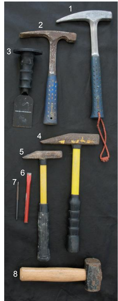
Figure 2.18 Some of the different geological hammers and cold chisels available on the market. (1) Estwing pick end hammer, (2) Estwing chisel end hammer, (3) cold chisel with hand guard, (4 and 5) 2.5 lb and 1 lb geological hammers with fibreglass shafts, (6) pencil chisel, (7) tile scribe and (8) 3 lb lump hammer.
