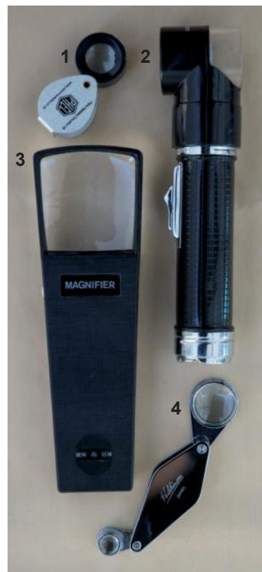
Figure 2.1 A variety of different hand lenses. (1) Standard 10× single lens; (2) 10× lens with built-in light – the lens casing matches the focal length; (3) 8× lens with built-in light; (4) 10× and 15× dual lens.
