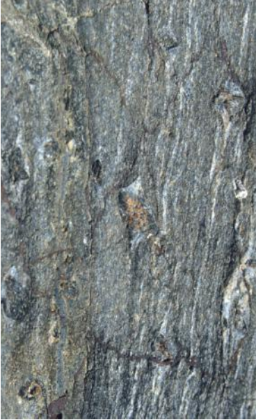
Figure 9.9 Pre-kinematic staurolite crystals strongly wrapped by a strong schistosity (orientated vertically). Some porphyroblasts (e.g. large crystal in centre) are flanked by strain shadows, mainly filled by a pale mineral. View about 7 cm across. (Tom W. Argles, The Open University, UK.)
