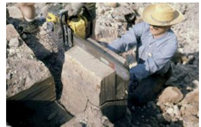
Figure 5.11 Cutting volumes of clays containing fossils using a carbide-tipped chainsaw. The advantage of this technique is that the samples can be taken back to the laboratory for detailed analysis. (Robert A. Spicer, The Open University, UK.)
