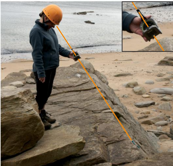
Figure 2.10 Measurement of the azimuth and plunge of a linear feature (slickenside lineations (Section 8.2.2)) on a fault plane using the sighting method with the Brunton-type compass-clinometer. Insets show detail of line of sight. The parts of the compass-clinometer are shown in Figure 2.3 a–c.
