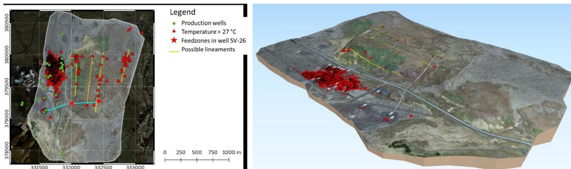
Figure 4: Temperature pixels (▲) hotter than 27 °C and a 3-D perspective draped on the 3 km<sup>2</sup> aerial photo
